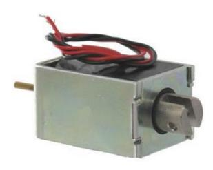
Stroke: 10 mm Force at beginning of stroke (FM: 100/40//25/5%): 1/2.5/5/8N Holding force power off: 30 N Power Consumption (FM: 100/40/25/5%): 6.5/20/40/65 W Total mass: 175 g Degree of protection / Energetic class: IP 40 / B Standard supplies: 24Vcc Possibles supplies: From 6 to 240Vcc Pulse duration: 100 à 150 Standard: NF C 79300 Examples of applications: various automations, multiple locks
