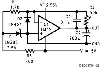
An op amp can be used as a positive or negative regulator. Unlike most regulators, it can sink current to absorb energy dumped back into the output. This positive regulator has a 0–50V output range.
