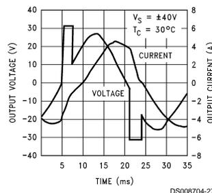
Should the power ratings of the LM12 be exceeded, dynamic safe-area protection is activated. Waveforms with this power limiting are shown for the LM12 driving  $\pm 26V$  at 30 Hz into 3Ω in series with 24 mH ( $\theta = 45^\circ$ ). With an inductive load, the output clamps to the supplies in power limit, as above. With resistive loads, the output voltage drops in limit. Behavior with more complex RCL loads is between these extremes.
