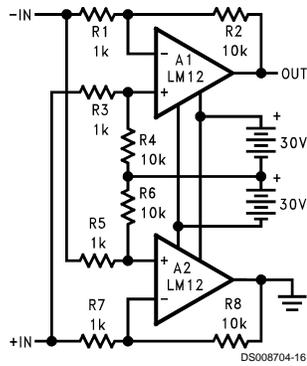
One limitation of the standard bridge connection is that the load cannot be returned to ground. This can be circumvented by operating the bridge with floating supplies, as shown above. For single-ended drive, either input can be grounded.
