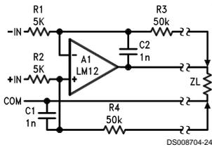
Remote sensing as shown above allows the op amp to correct for dc drops in cables connecting the load. Even so, cable drop will affect transient response. Degradation can be minimized by using twisted, heavy-gauge wires on the output line. Normally, common and one input are connected together at the sending end.
