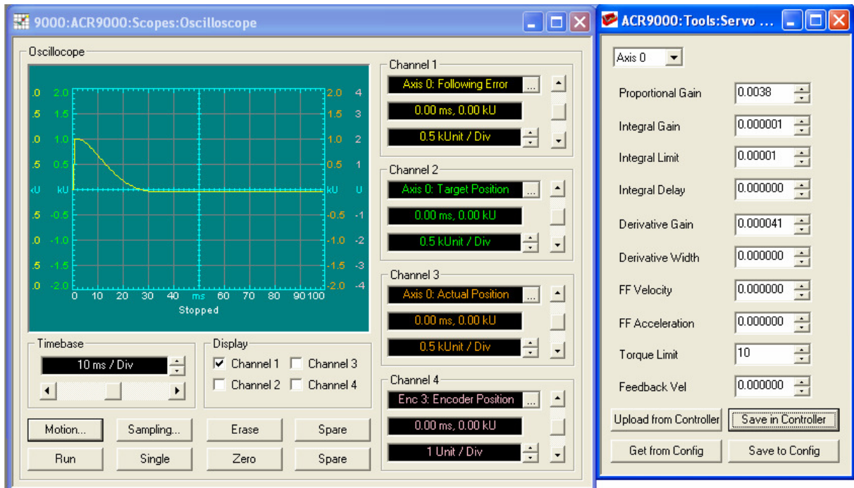
Example of a well-tuned T2D-4P (unloaded), settling within 30ms
