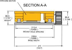
LIMIT LOCATION DEPENDENT ON COMPRESSED BELLOWS LENGTH REFER TO TRILOGY WEB SITE 96.3 [3.793] or 66.3 [ 2.612 ] FIRST MOUNT HOLE 0 Ó 0 Ó 0 Ţσ 0 6 0 0 0 CARRIAGE LENGTH 0 OAL 0 6 В В 0 0 0 000 0 c 0 a 6 0 C 120.0 [ 4.724 ] TYPICAL POSITIVE DIRECTION OF TRAVEL
