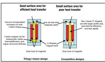
What results is a compact motor design with high force and extraordinary thermal characteristics.
