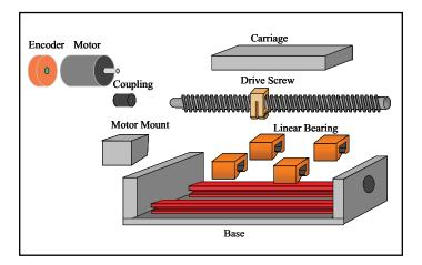
Fig. 1: Precision table fitted with ballscrew drive
