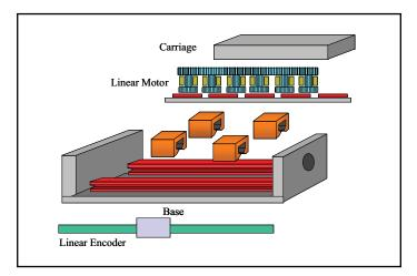
Fig. 2: Precision table fitted with linear motor
