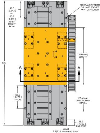
TRAVEL (mm) = OAL - 66.0 - CARRIAGE LENGTH OVERALL LENGTH (OAL) = MULTIPLE OF 60 mm UP TO 4080 mm
