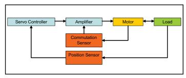
Fig 16(b): Servo Motor Control (position sensor located at load)
