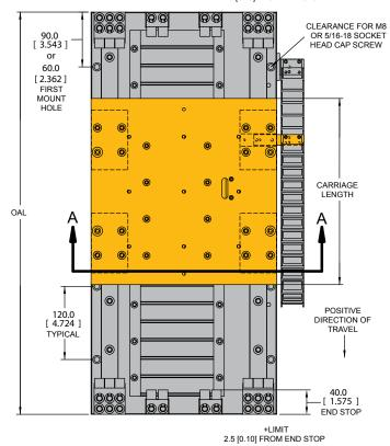
TRAVEL (mm) = OAL - 80.0 - CARRIAGE LENGTH OVERALL LENGTH (OAL) = MULTIPLE OF 60 mm UP TO 4080 mm
