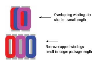
Fig. 9: Overlapping Windings
