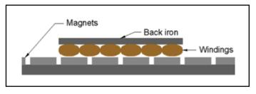
Fig. 13: Slotless Linear Motor
