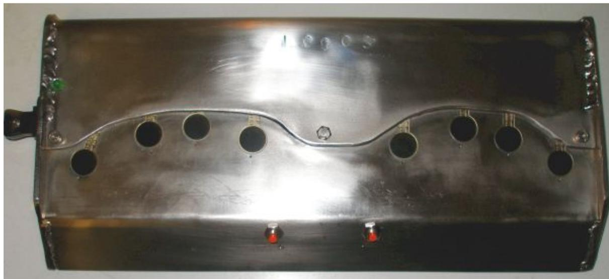
The power supply connector as well as the midi-out socket are on the left of the pressure pad console. All circuitry fits nicely underneath inside the console.
