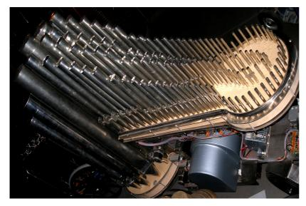
With its 145 pipes,  $\langle Qt \rangle$  could barely become a light instrument. Although it weighs over 270 kg, it is easily transportable using its own sturdy and flexible wheelbase. The wind chest was split into two section to achieve compactness and to limit building height. The two tremulant rotating valves in the wind supply channels are driven by stepper motors. Wind pressure for  $\langle Qt \rangle$  is 14mBar and can be modulated.
