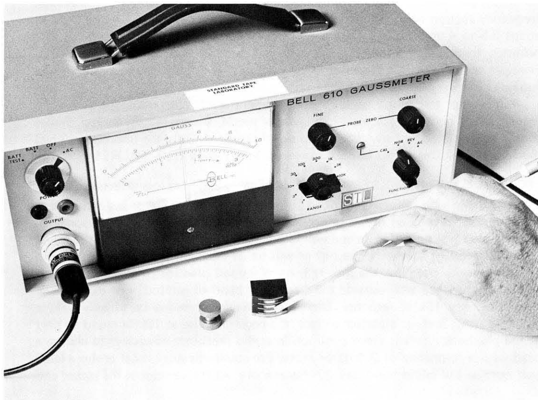
Hall effect Gaussmeter – Note: Head shows almost 5 Gauss field.
