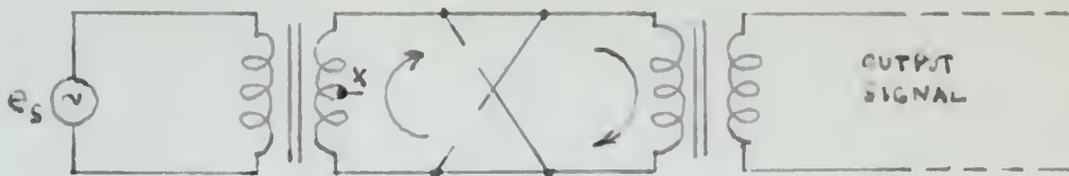
Equivalent Circuit During Negative Half Cycle
