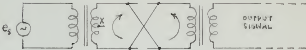
Equivalent Circuit During Positive Half Cycle
