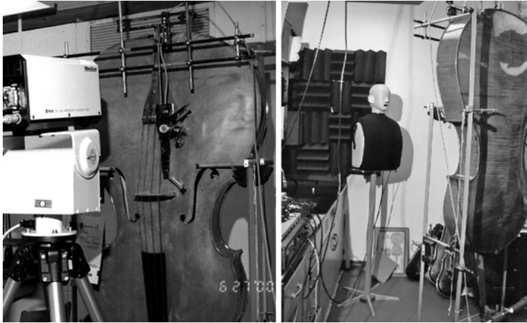
Fig. 18.4 Small bass in testing support fixture. Vibration measurements: force hammer impact excitation; scanning laser vibration response measurement ( left ). Room-average acoustic measurements: excitation and support as for vibration, but with acoustic measurement corner setup using dual microphones in sound quality head ~1.5 m distant from instrument ( right )
