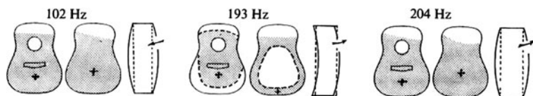
Fig. 3.10 Vibrational motion of a freely supported Martin D-28 folk guitar at three resonances in the low-frequency region (Fletcher and Rossing 1998)
