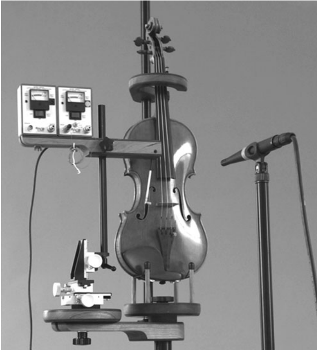
Fig. 13.11 Apparatus for measuring sound radiation using an impact hammer. It can be set up in a violin maker's workshop
