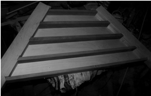
Fig. 21.6 The interior braces of a hammered dulcimer terminate at the pin block and may be modeled as simply supported (hinged at the end) beams. The end rails will be glued to the top and bottom braces. Because they extend across the entire pin block, they can be modeled as clamped beams
