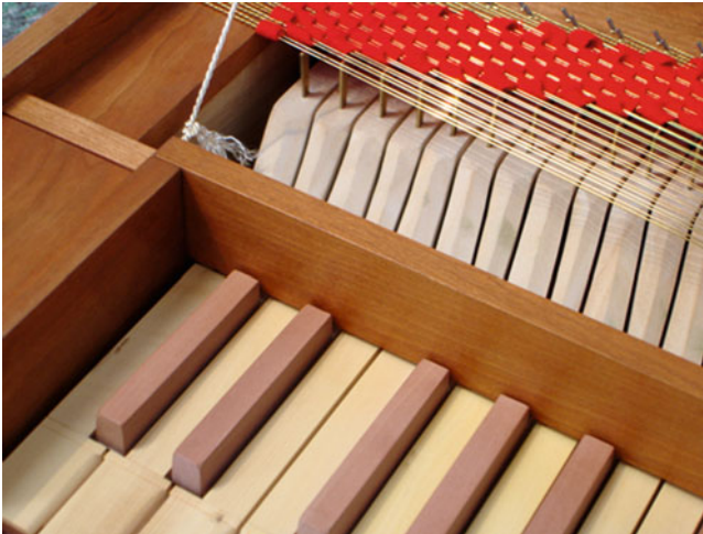
Fig. 8.10 Detail of action of the reproduction Hubert clavichord. Each key is pivoted on the balance rail and, when it is depressed, the brass tangent at its distal end strikes the pair of strings corresponding to that note. The listing cloth is clearly visible
