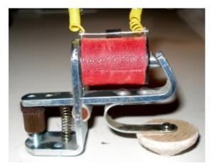
Thanks to these valves, we obtained velocity sensitivity for each individual note as well as individual key pressure modulation (note aftertouch). The sizing of the pallet valves with conical pads is given in the table above. These sizes were calculated such that for a given solenoid trajectory (5 to 10mm) and orifice, flow regulation is optimal. We designed software to calculate the
