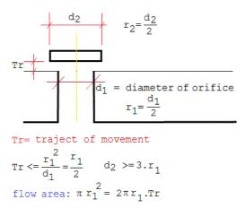
The results prove the superiority of conical valves but also make clear that for trajectories in the order of 4 to 8 mm, the use of conical valves on very large orifices would not be appropriate. For instance, they would not have been a good choice on the lowest pipes of our <Qt> robot.
