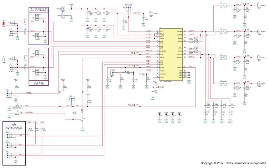
Figure 4. TPA3129D2EVM Schematic
