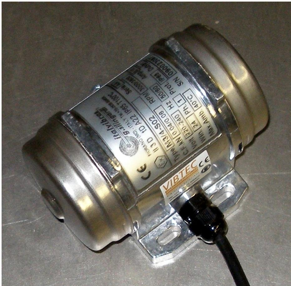
The model shown on the picture weighs 850 g and has a power rating of 20 W. It is very quiet in operation. For variable frequency use, we advise using them with an amplified sine wave. Make sure the voltage is reduced when the frequency goes down. If a 3-phase motor has to be steered, following circuit gives good performance over a wide frequency range, in fact only limited by the possibilities of the motor::
