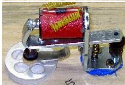
The types shown on the pictures are made by August Laukhuff: the left one has a 35 mm pallet, the right one 40 mm. These types can easily be converted to operate conical valves by exchanging the flat pallets with conical ones, as shown in the first picture under this heading. For good velocity control, the original springs must be replaced with a stronger type. Details can be found in our pages on the development of our 6-octave quartertone organ <Qt>.
