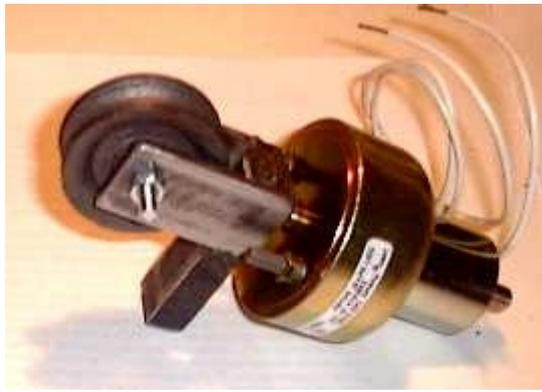
Note that these soft-shift magnets, although extremely expensive, are devices that respond relatively slowly. The forces involved here preclude the use of moving coil mechanisms. Pneumatic cylinders would be ideal here, if they didn't suffer so much from exhaust noises...
