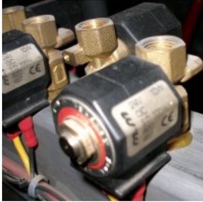
Solenoid valves can be operated either on AC or DC, but for automated instrument use, only DC should be considered, since when driven with AC you will get a 50Hz buzz enriched with overtones from each of them...
