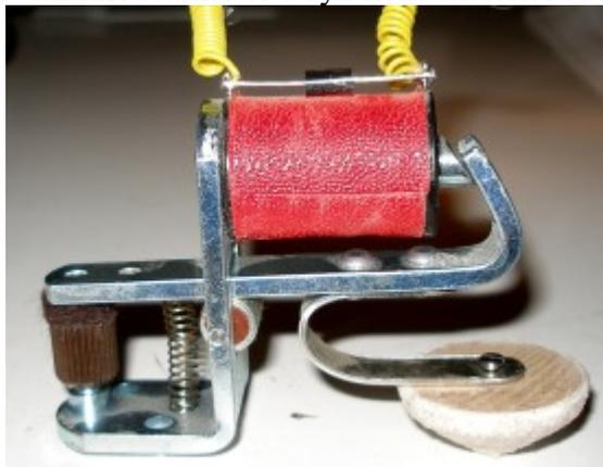
Conical valves can also be operated with tubular solenoids. As an alternative, moving coil valves, which can be made from re-engineered loudspeakers, can be used as well. In the latter case they can be driven with bipolar analogue DC
